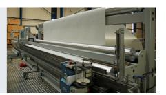
This kind of machine is suitable for rewinding rollers up to a width of 5.000 mm, max roller diameter of 1.200 mm and a max speed of 300 m/min.
